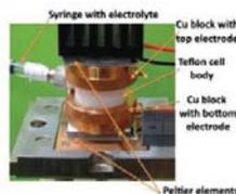
Home-made thermoelectric cell with Glassy carbon electrodes
